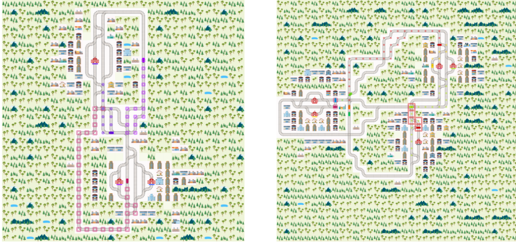
Figure 4: Two environment states with the respective visited cells in the observation for each agent highlighted, with so called “demo” setup (5 agents, left) and “mini” setup (20 agents, right). Note how as agents on the map raise in numbers, the traffic increases and deadlocks start to occur.
