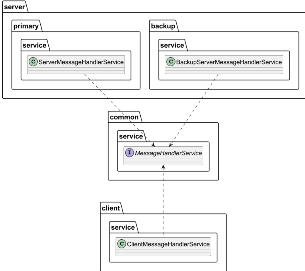
Figure 6: Class diagram focused on the common interface and implementations of the Message Handlers.
